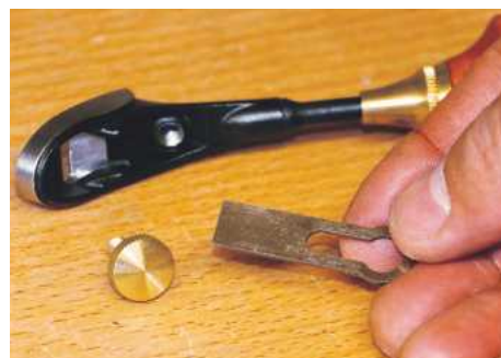
▲ You have to remove the retaining knob to hone the iron
